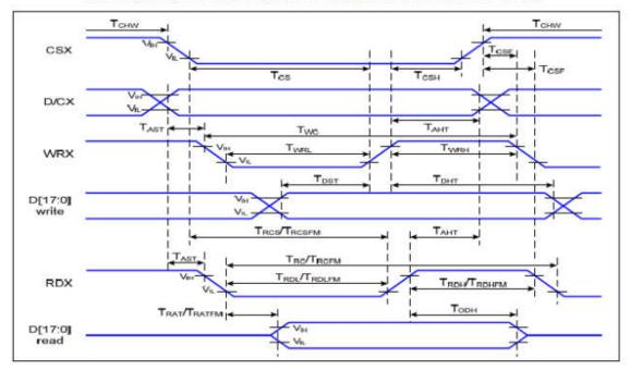
Parallel Interface Timing Characteristics (8080-Series MCU Interface)
