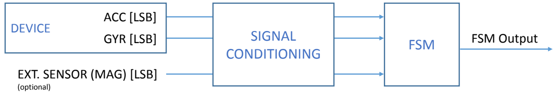
Figure 2. State machine in the LSM6DSOX
